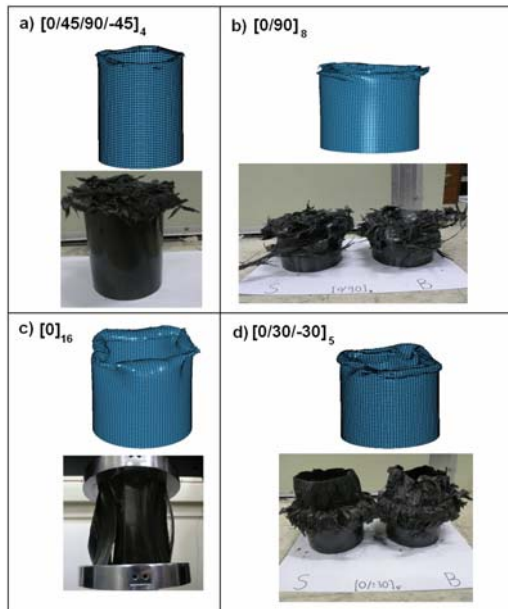
Fig. 14 Final stage of the specimens (S: notch, B: bevel).
