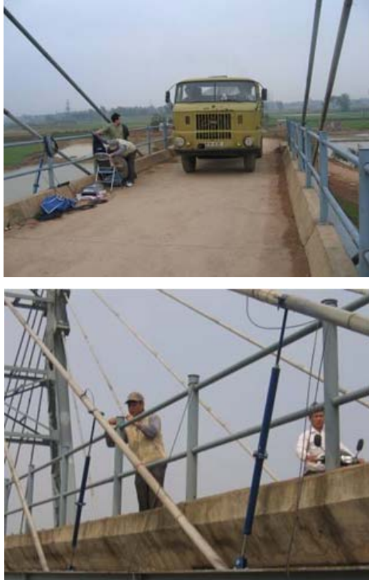
Figure 11. Damper-cable experiment in Ben Coc Bridge
