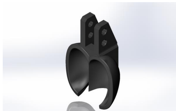
Figure 5. 3D layout of Pelton bucket
