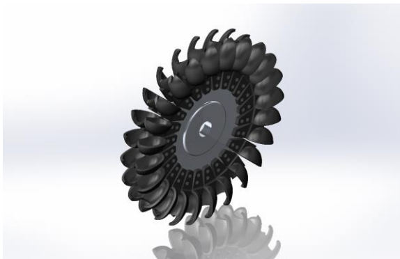
Figure 7. Pelton turbine runner with 24 buckets
