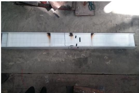
Figure 10 – Crack image of the steel beam sample with pre-crack on the bottom side of beam at the middle of span – Type 2.
