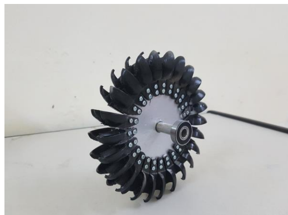
Figure 19. Photograph of Pelton turbine runner
