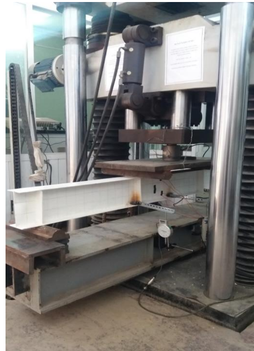
Figure 2. Bending test of steel beams
