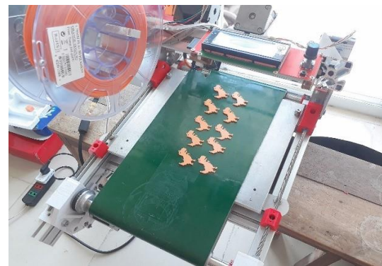
Figure 24. Multiple objects print test
