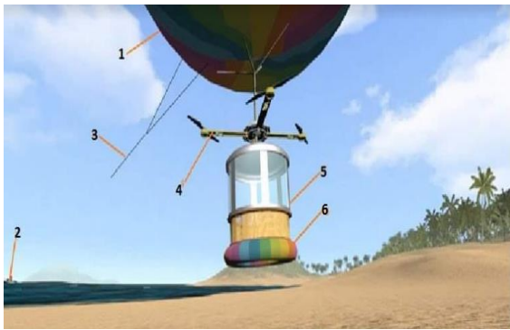
Figure 1.1. The airship for tourism of new scheme: The sphere with light gas (helium gas) (1) pulled by a vessel (2) via the smart winch and towing system (3), a quadrotor/ multirotor (4) is hung under the sphere and is connected with passenger compartment (5), a safety toroidal airbag (6) is connected at the bottom.
