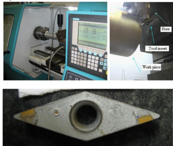
Figure 1. Turning experimental test
